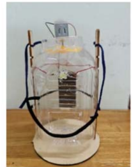
Figure 2: Hands-on makers' activity - designing and producing an electrical product applying the parallel circuit from recycled material
